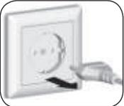
Remove the mains plug from the socket and the small appliances plug from the RolloTron Standard swivel winder.
