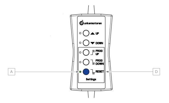
If the drive is mounted in the blind it is recommended to run the blind to the desired lower end position before reestablishing the delivery state.
